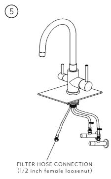
Connect cold line associated with filter handle to filter hose connection
